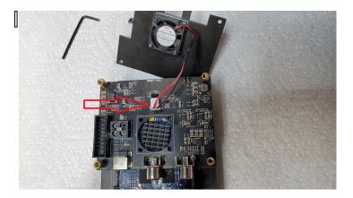
2.10. Align the rear panel over the PSU16 board and ensure the fan wires are routed to the right of the fan footprint so wires are not pinched between the fan and the PSU16 board.
