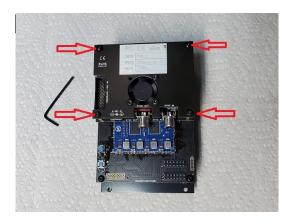
2.3. Unplug fan wires from fan plug header on PSU16 board.
