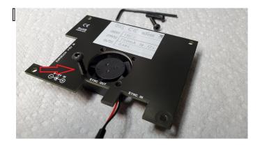
2.7. Hold the fan while using the included 2mm allen wrench to drive the screw into the fan housing. There will be some friction as the screw cuts its threads into the plastic fan housing.
