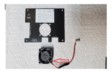
2.6. Line up the rear panel fan mounting holes over the fan and twist in one mounting screw just enough to hold the screw. Ensure the screw is perpendicular to the rear panel.
