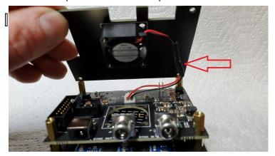
2.11. Reinstall rear board onto unit and fasten the four allen head screws.
