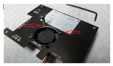
2.9. Once the fan is installed on the rear panel. Plug the fan connector into the fan header pins on the core board. Orient the fan connector so the Red wire is on the left pin as shown in the picture.
