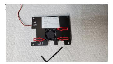
2.5. Remove the old fan. Align the new fan so the fan wires are oriented to the bottom right as shown in the picture.
