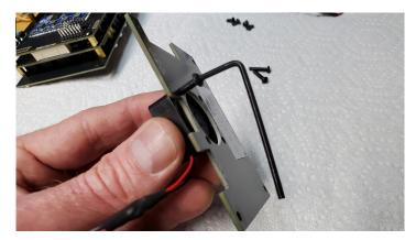
2.8. Install the remaining fan mounting screws. Do not over tighten.
