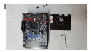
2.4. Using the included 2mm allen wrench, remove the 2mm allen head screws holding the fan to the rear board.
